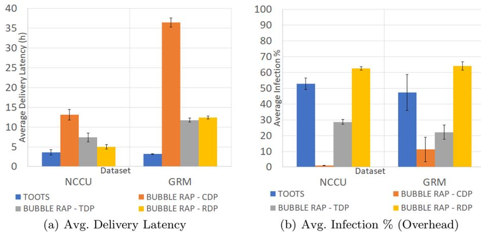
**Fig. 5.** Delivery Latency and Overhead Performance Comparison of TOOTS, Bubble Rap-CDP, Bubble Rap-TDP, and Bubble Rap-RDP on NCCU and GRM datasets.
