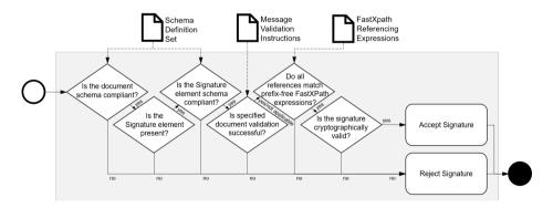
Fig. 5: Guideline for XML Signature Verification
