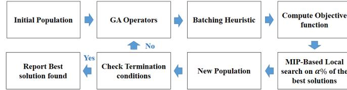
Fig. 1. Schematic pattern of proposed Matheuristic algorithm
