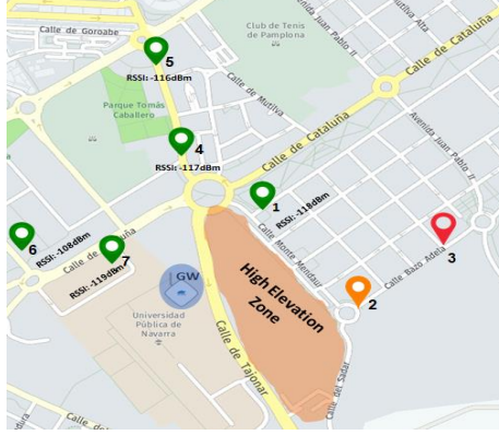
Fig. 4. LoRaWAN measurements results. Green: No packet losses. Yellow: some packet losses. Red: All packets lost.
