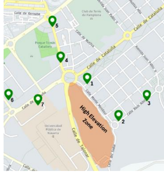
Fig. 5. SigFox measurements results. Green: No packet losses. Yellow: some packet losses. Red: All packets lost.
