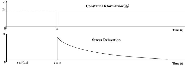
**Fig. 3.** Stress relaxation of a viscoelastic material after a step displacement.
