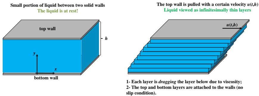
**Fig. 1.** Illustration of a Couette flow. A certain velocity  $u(t, h)$  is imposed at the resting upper wall. As this wall moves along time, the displacement information travels along the different layers of fluid until it reaches the bottom wall. Note that these layers are merely illustrative.
