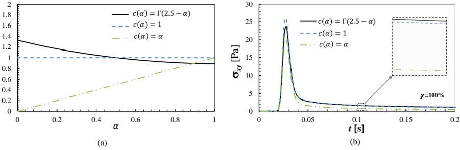
**Fig. 5.** (a) Three different functions  $c(\alpha)$ . (b) Stress relaxation test in a narrow gap Couette cell following a sudden straining deformation (the upper wall moves) for  $\gamma_0 = 100\%$  and different functions  $c(\alpha)$ .
