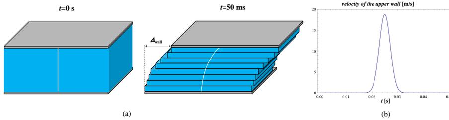
**Fig. 4.** Step displacement. (a) Initial and final state of the deformation. After 50 ms the upper wall stops moving (the displacement is  $\Delta_{wall}$ ). (b) Variation of the upper wall velocity along the 50 ms. The deformation ( $\gamma_0 = \Delta_{wall}/h$ ) is 100%,  $\psi = 0.003$  and the delay ( $t_d$ ) is 0.025 seconds.
