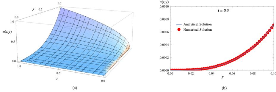
**Fig. 2.** (a) 3D plot of the analytical solution given by  $u(t, y) = t^{1/2}y^3$ . (b) Comparison between the analytical and numerical solutions for  $h = 0.1$ ,  $t = 0.5$ ,  $\Delta\alpha = 0.1$ ,  $\Delta t = 0.01$  and  $\Delta y = 0.002$  ( $\varepsilon_{\Delta t, \Delta y} = 1.40337 \times 10^{-6}$ ).
