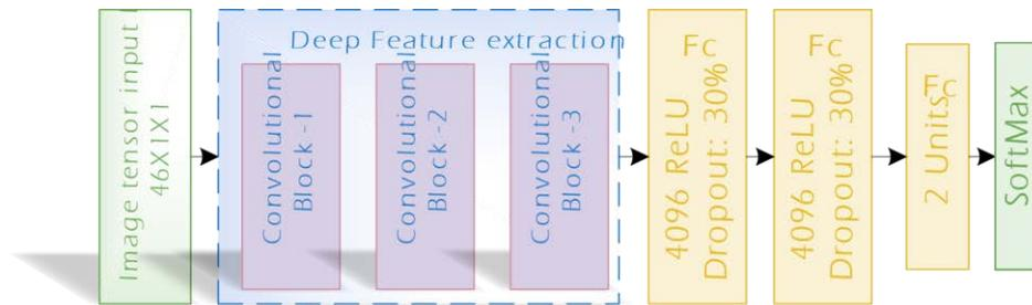
Fig. 8.2. CNN Architecture, first block: input layer. Second: convolutional deep feature extraction module. Third and fourth: Fully connected plus ReLU layer and dropout. Last two layers, fully connected layer and SoftMax layer.
