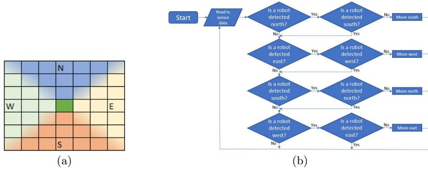
**Fig. 1.** Distributed area coverage solution: (a) The agent (in centre) has four contact sensors (not shown) and four optical sensors, with the respective field of view indicated (bi-coloured cells are within the range of multiple sensors). Here the range of the optical sensors is of length three. (b) Flowchart for the memoryless coverage controller.
