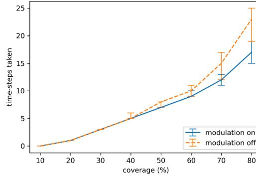
**Fig. 3.** Comparison of the time taken for different levels of coverage to be achieved with sensing range modulation on vs off. Runs for different levels of coverage are independent. Error bars indicate the range.
