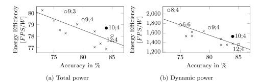
Fig. 3: Total and dynamic energy efficiency on the ZCU102 in relation to the accuracy. Pareto optimal configurations are shown as circles and are labeled with the quantization level. A trend line indicates the correlation between the efficiency and the accuracy.
