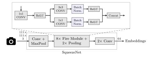
Fig. 1: Overview of our SqueezeNet, changes are highlighted by a dashed pattern.
