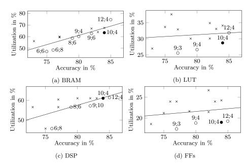
Fig. 2: Utilization of BRAMs, LUTs, DSPs and Flip-Flops of the ZCU102 in relation to the accuracy. Pareto optimal configurations are shown as circles and are labeled with the quantization step: The first and latter number represents the fraction bit width of weights and activations, respectively. A trend line indicates the correlation between primitive utilization and accuracy.
