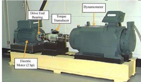
**Fig. 4.** Experimental set up by Case Western Reserve University[33].
