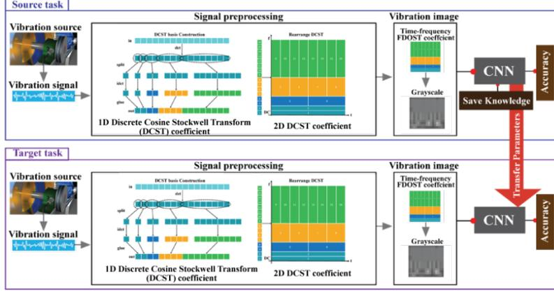
Fig. 1. The block diagram of proposed approach.
