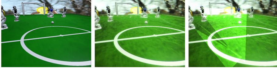
**Fig. 2.** After changing the background in the simulated image to a random image from the COCO dataset (left), we apply the image-to-image translation learned by MUNIT to it (middle). In addition to the offline augmentation obtained with the sim-to-real translation, we perform an online augmentation during training (right). Beside standard augmentations such as blur, we also introduce a simple simulation of sun light patches on the field.
