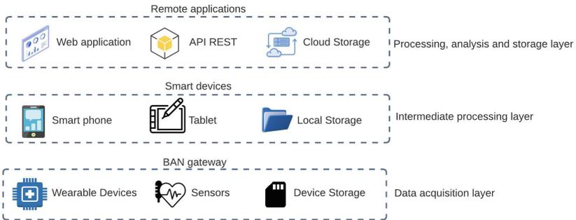
**Fig. 1.** Three-layer HMS architecture. adapted [3].
