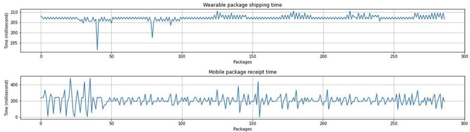
**Fig. 4.** Package exchange time between wearable system and mobile app.
