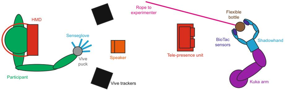
**Fig. 1.** Schematic overview of the setup, with equal colours indicating systems that were synchronized between participant on the left and remote robot on the right. The Kuka arm was set in a convenient fixed position, so only the Shadowhand reacted to the user’s motion (for clarity, only 2 of the 5 fingers of the Shadowhand are shown). A rope, attached to the bottom of the water bottle, was lead through a pulley underneath the bottle, and lead back to the experimenter for slip induction.
