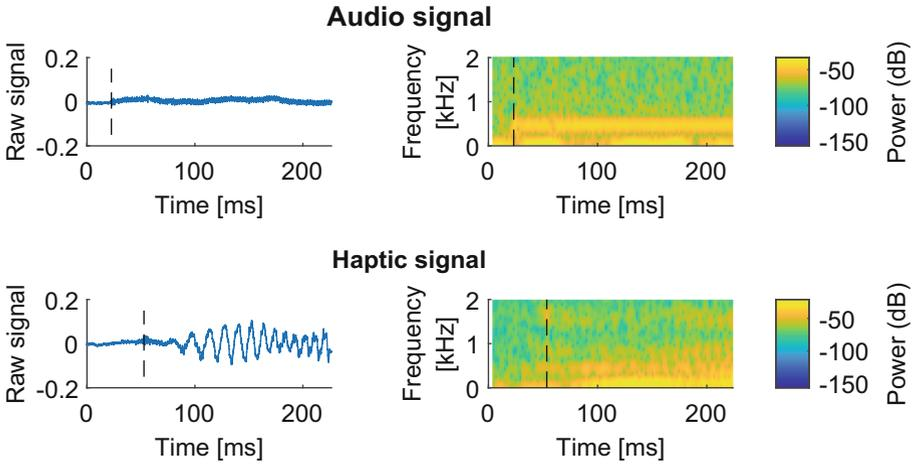
**Fig. 2.** Recordings from stereo contact microphones to test onset latencies between haptic and auditory stimuli. Left column: raw recordings, right column: spectrograms. The vertical dashed lines indicate determined onset times. For this recording, the measured haptic signal lagged the auditory one by 30 ms. Note that the measurement is only meant to determine the difference in onset times, so  $t = 0$  has no specific meaning.
