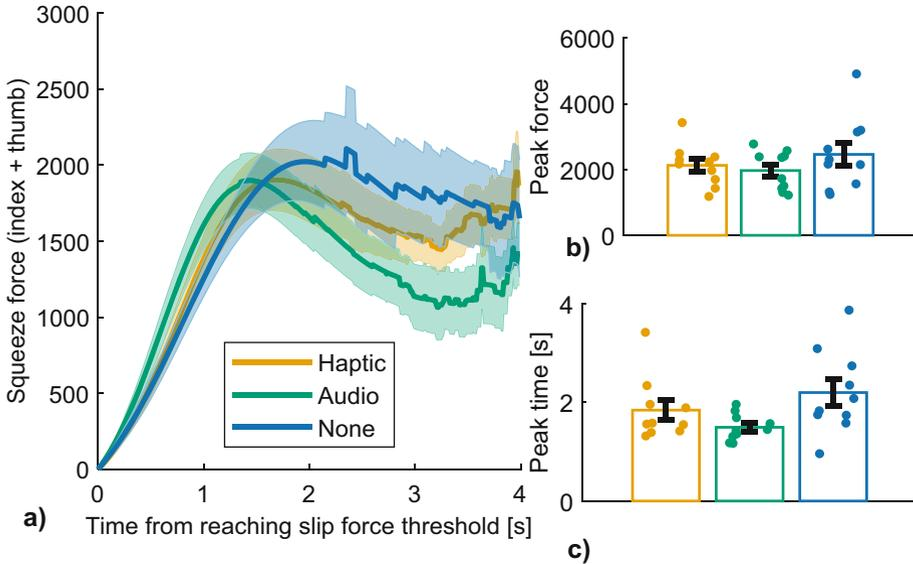
**Fig. 3.** Squeeze forces (mean  $\pm 1$  standard error), as measured at the remote robot’s fingers. (a) Average time traces (solid lines) across participants. Time = 0 represents the time at which the slip threshold was passed. (b) and (c) Times and heights, respectively, of the squeeze force peaks, with one marker per participant.
