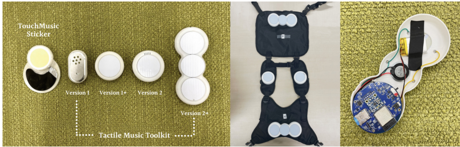
Fig. 1. (left) Various Furekit modules; (middle) attached to a wearable vest; (right) custom board fitted into a Furekit
