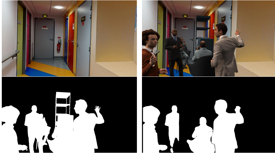
Fig. 3. The example of the query image and masks. The top left image is a query image without any moving objects. The top right image is a dynamic query with added objects. The bottom left image shows the ground truth masks of the added objects. The bottom right image shows the result of our instance segmentation using YOLACT.
