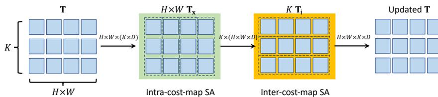
Fig. 2: Alternate-Group Transformer Layer. The alternate-group transformer layer (AGT) alternatively groups tokens in  $\mathbf{T}$  into  $H \times W$  groups that contains  $K$  tokens ( $\mathbf{T}_x$ ) and  $K$  groups that contains  $H \times W$  tokens ( $\mathbf{T}_i$ ), and encode tokens inside of groups via self-attention and ss self-attention [8] respectively.
