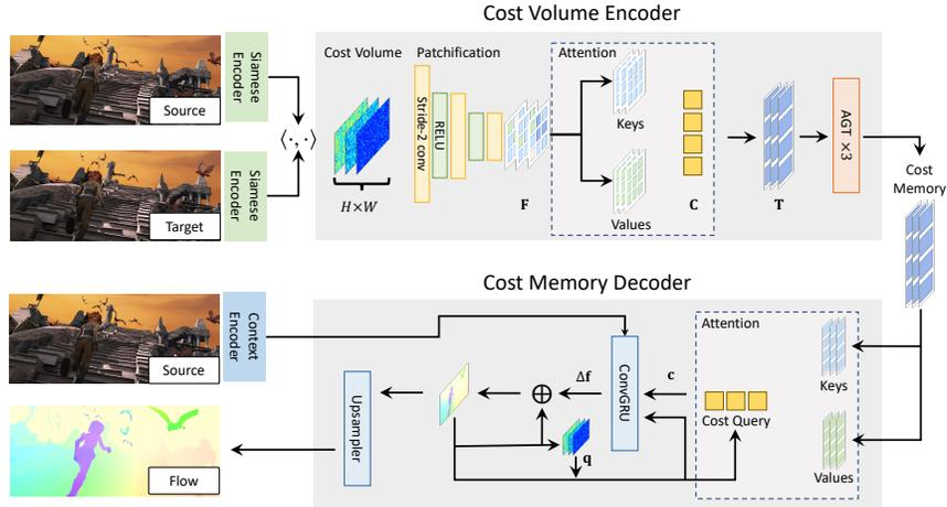
Fig. 1: Architecture of FlowFormer. FlowFormer estimates optical flow in three steps: 1) building a 4D cost volume from image features. 2) A cost volume encoder that encodes the cost volume into the cost memory. 3) A recurrent transformer decoder that decodes the cost memory with the source image context features into flows.
