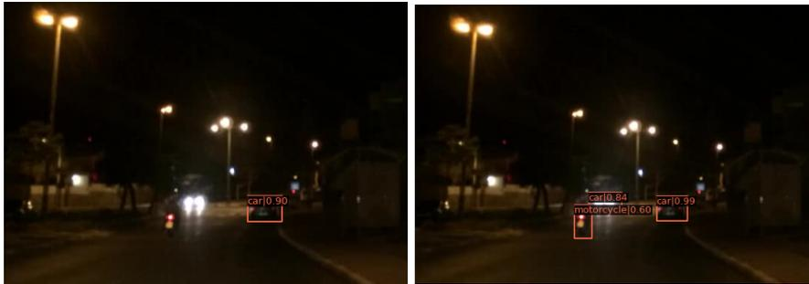
Fig. 9: A false negative motorcycle at night (left) fixed to a true positive detection (right) using TALISMAN.
