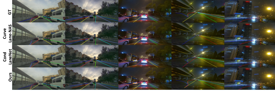
Fig. 7. Comparison of visualization results between our RCLane and other lane detection methods. Our method performs better in different scenarios such as occluded, curved and Y-shape lanes.
