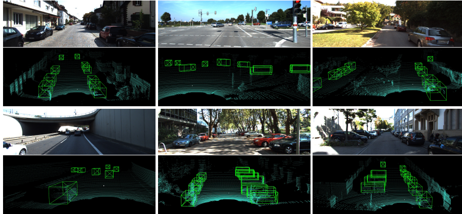
Fig. 5. Snapshots of qualitative results on KITTI test set. The output 3D bounding boxes are shown in green.
