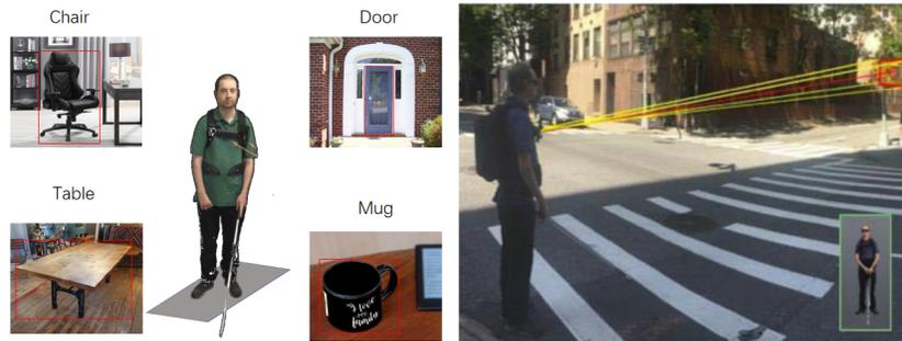
Fig. 1: Challenges for pBLV exist in various scenarios: Searching for objects of interests and walking to the objects (Left). Our wearable system contains a backpack with a monocular camera, an Nvidia Jetson Xavier NX Developer kit, and battery. The camera is placed on the chest of the user (Right).
