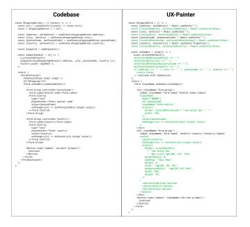
**Fig. 4.** Comparison of the application's codebase against the code generated by UX-Painter. Green lines correspond to the changes imposed by refactorings.
