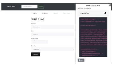
**Fig. 3.** ReactJS component generated for the alternative version. The user can observe a preview before downloading it.
