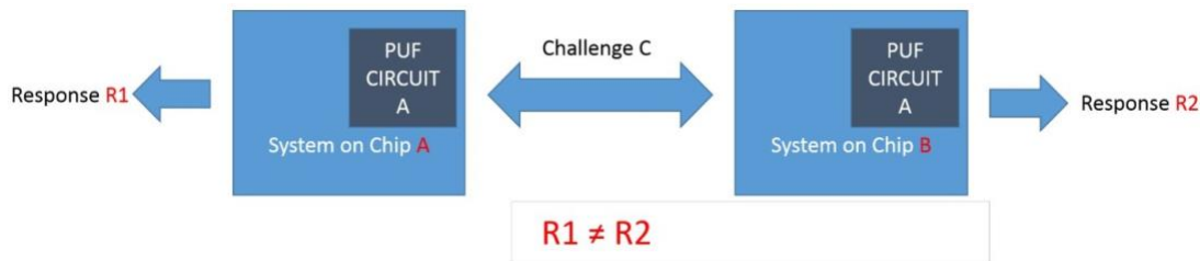
Figure 3. Response produced on PUF circuit of two different ICs [12].
