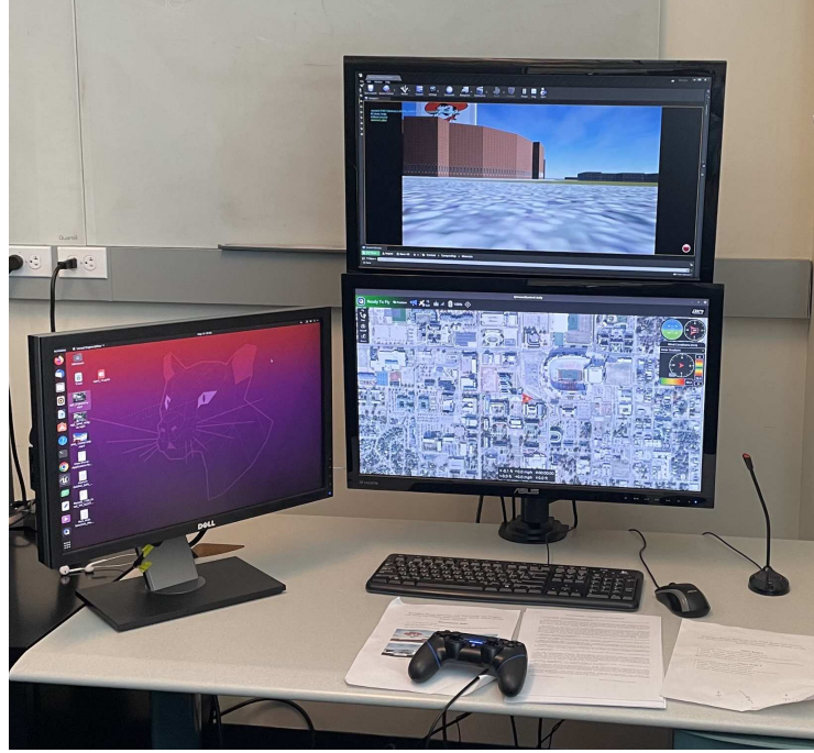
Fig. 3: Experimental setup: upper screen shows the environment and the lower screen shows the ground control station. Participants are also required to use the mouse and the joystick.
