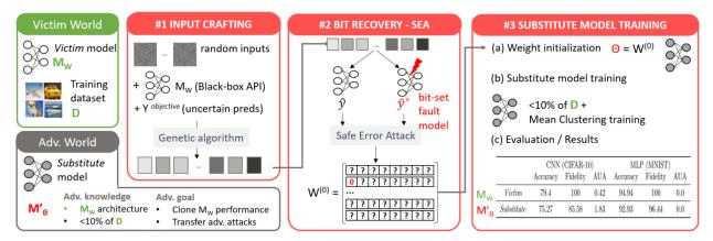
Figure 1: The adversary crafts inputs and performs a safe-error attack exploiting faulted predictions with bit-set fault injections on the parameters stored in memory. The objective is to partially recover the bits of the parameters to efficiently train a substitute model that mimics the victim model with high fidelity.
