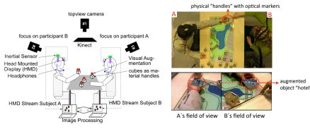
such as three DV cameras, a Microsoft Kinect and two to three workstations. Each participant also wears a head-mounted display, a microphone headset and a BRIX motion sensor to measure head movement at high temporal resolution.
