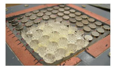
**Fig. 1.** Image of the bristles fabricated to emulate natural cilia. This design is used as an alternative to the membrane design described in [13]
