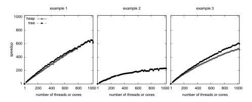
**Fig. 5.** Speedup of the DMPMC algorithm on a cluster of 64 nodes (a total of 1024 cores) interconnected with a QDR InfiniBand network. The coefficients of polynomials are quadruple precision floating point numbers.
