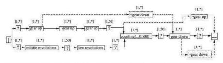
Fig. 1 Example of a pattern graph describing a driving cycle (learned from data, see [10])
