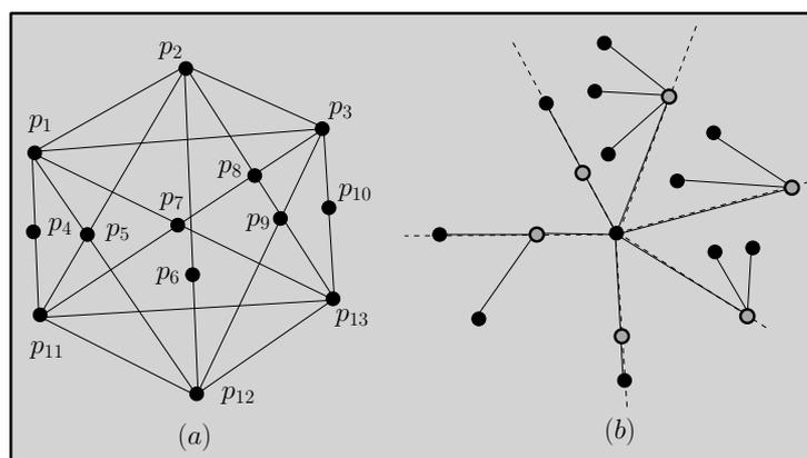
Figure 10: (a) A PVG with  $A = \{p_1, p_2, p_3\}$ ,  $B = \{p_4, p_5, p_6, p_7, p_8, p_9, p_{10}\}$  and  $C = \{p_{11}, p_{12}, p_{13}\}$ . (b) Points of A and C connected by edges representing blockers.
