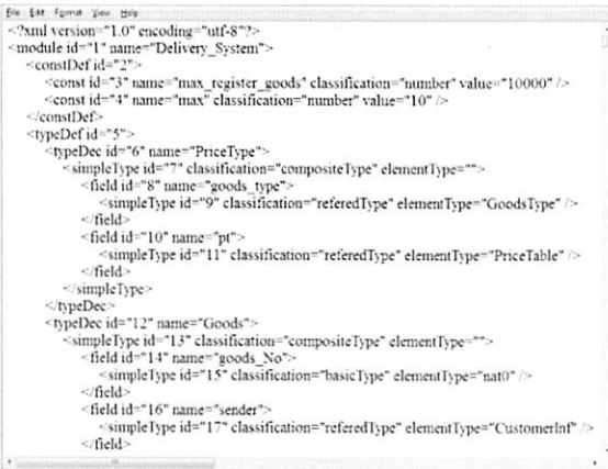
Fig. 12. The figure shows the main output of this tool: xml file storing syntax information and functional scenarios.
