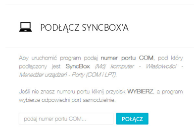
Fig. 5. The screenshot of the interface for connecting Arduino with SyncBox; PODŁĄCZ SYNBOXA - connect SyncBox. The user can start using the system by clicking one button, POLACZ (connect).
