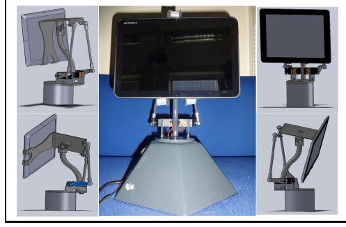
Fig. 1. Embodied Telepresence System (ETS) Actual Design and CAD Model
