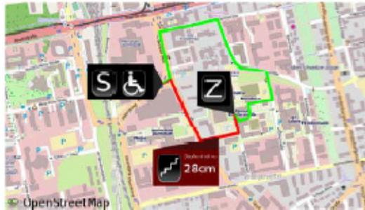
**Fig. 4.** Display of a barrier (staircase with steps of 28cm height) along a selected route (red) and computed barrier-free detour (green)
