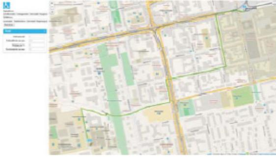
**Fig. 12.** Computing and drawing a route based on a profile which allows 1 step (German: Stufenanzahl), widths of 735 cm (German: Rollstuhlbreite in mm), an incline gradient of 6% (German: Steigung in %), and curb heights of 30 mm (German: Bordsteinhöhe in mm)
