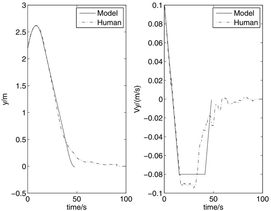
**Fig. 3.** The performance of one of experts in the simplified RVD task with initial condition 1. Left: position deviation. Right: velocity deviation. Solid line: model. Dash-dot line: human operator.
