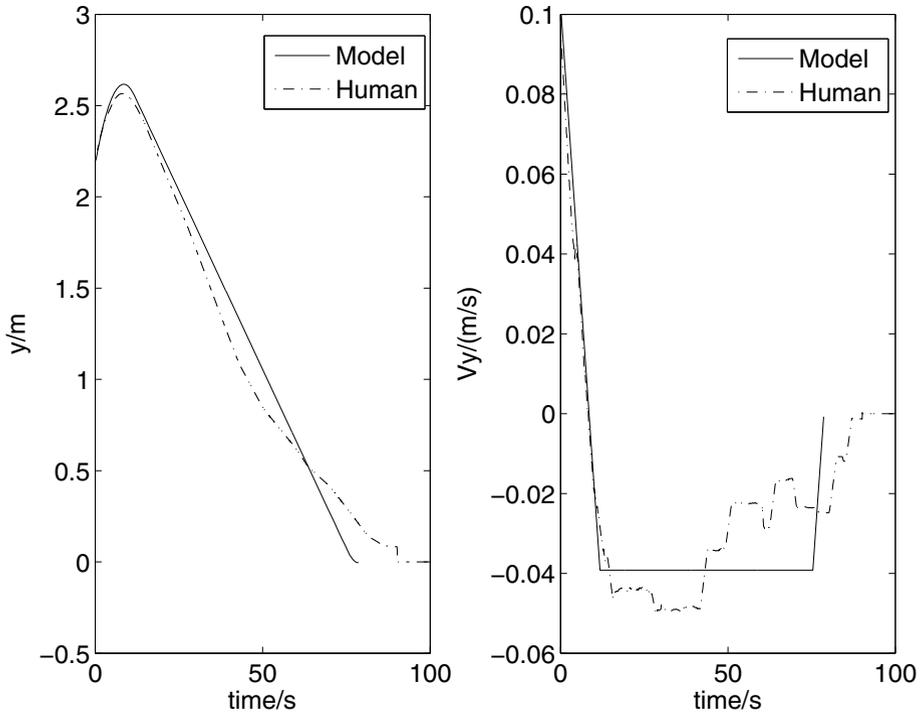
**Fig. 4.** The performance of one of less-skilled participants in the simplified RVD task with initial condition 1. Left: position deviation. Right: velocity deviation. Solid line: model. Dash-dot line: human operator.
