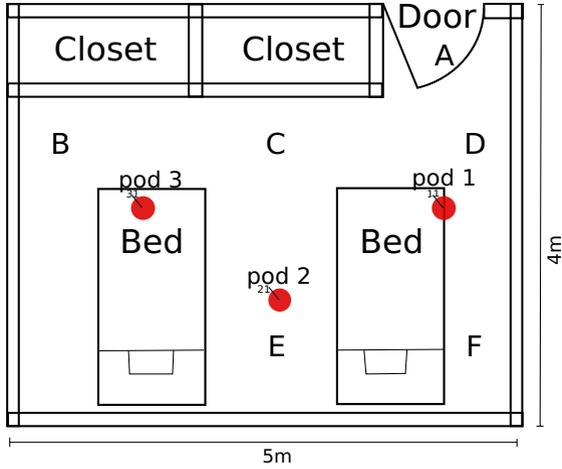
**Fig. 2.** Room details and sensor pod positioning
