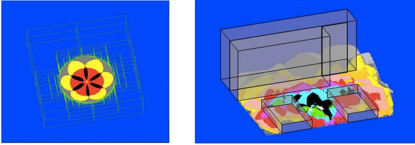
**Fig. 4.** Left: coverage area of a single sensor pod. Right: combined coverage area of a room with three sensor pods.
