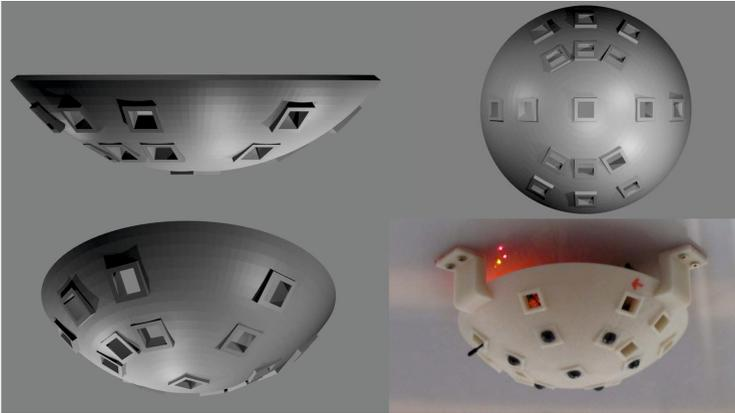
**Fig. 1.** The sensor pod design and the final 3D printed prototype
