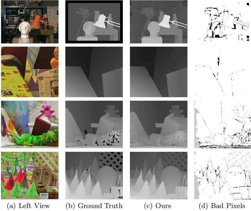
**Fig. 3.** Our results on the four online testing images of Middlebury. The error maps shown in the last column are evaluated at 0.5 error threshold.
