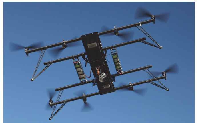
Figure 1. Octocopter HORUS with bottom mounted camera
