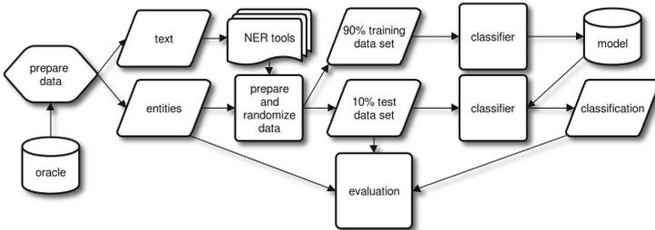
**Fig. 1.** Workflow chart of the evaluation pipeline
