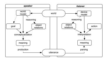
**Fig. 2.** Schematic of the systems involved in autonomous processing of spatial scenes such as the one shown in Figure 1. Left are the processes the speaker runs, in order, to produce an utterance. Right shows the processes the hearer is running for understanding a phrase.
