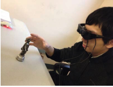
Fig. 1. A user is grasping an object, while the grasp is recorded by the egocentric stereo cameras
