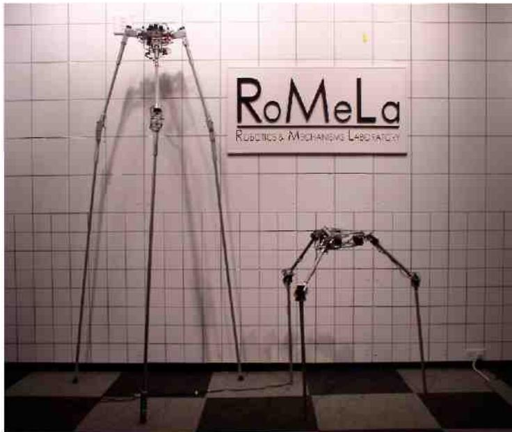
**Figure 3.2:** The RoMeLa STriDER has a unique tripedal locomotion that is stable and agile while walking.
