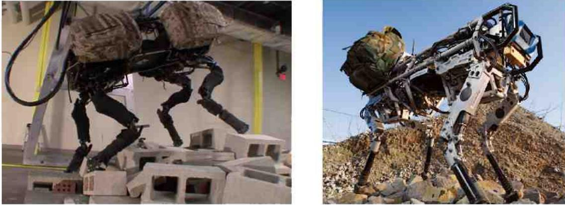
**Figure 2.4:** BigDog robot can walk across rubble, climb hiking trails and walk in snow and water.
