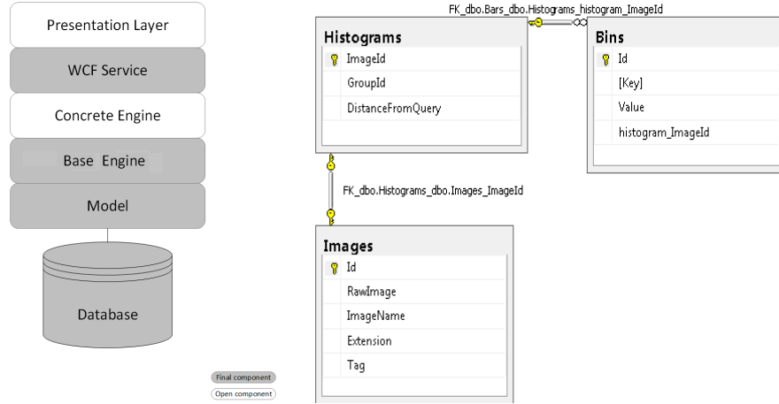
(a) Multi-tier architecture for storing visual data. Final components are compiled release of dll's and open components are user implementation. (b) Entity diagram based on database tables.
