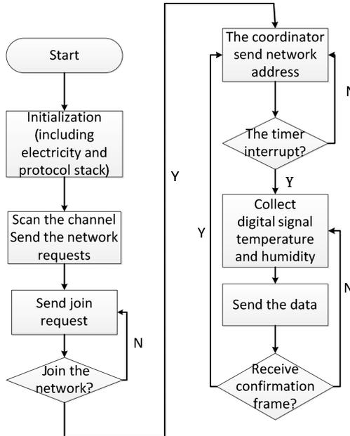
Fig. 10. Flow chart of acquisition node
