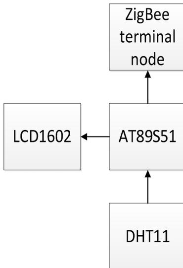
Fig. 2. Block diagram of system structure.
