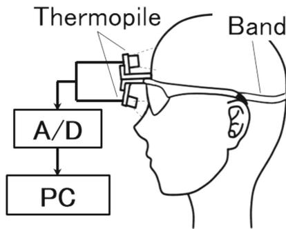
**Fig. 2.** Developed glasses-like wearable nasal skin temperature measurement device
