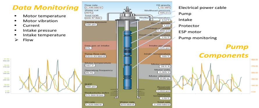
Fig. 1. Electric Submersible Pumps (ESPs)
