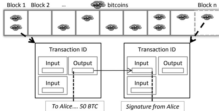
**Fig. 1.** Transactions stored on the Blockchain based on [19]
