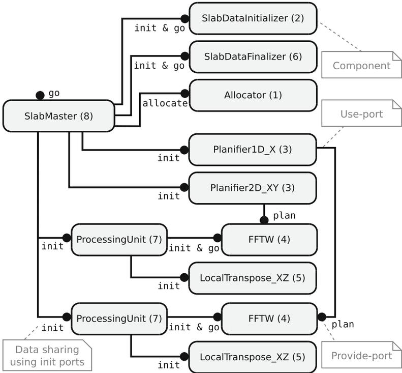
**Fig. 1.** Local (one process) basic 3D-FFT assembly using 1D decomposition.
