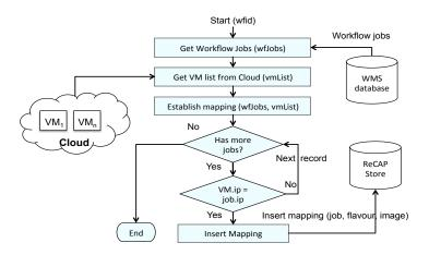
Fig. 2. Flowchart of the job to the Cloud resource mapping in the Static environment
