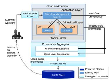
Fig. 1. General overview of the ReCAP architecture
