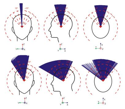
**Fig. 1.** Angular orientations in frontal, sagittal and transverse planes measured with the ENLAZA interface. Above, an individual without motor disorders; below, one with CP.
