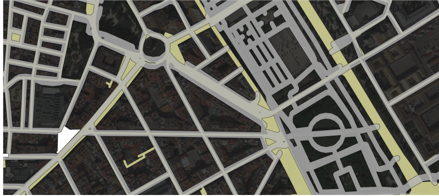
Fig. 4 Polygon-based approach for integrating UA and OSM datasets: white lines represent OSM line features, with buffered by a chosen distance (grey), white polygon represents OSM pedestrian area; green polygon comes from UA dataset of land use type 'Roads and associated land'
