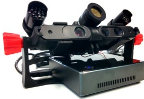
Fig. 1. Eye tracker setup with high resolution Flea3 camera, Asus Xtion, IR Led clusters and processing unit.
